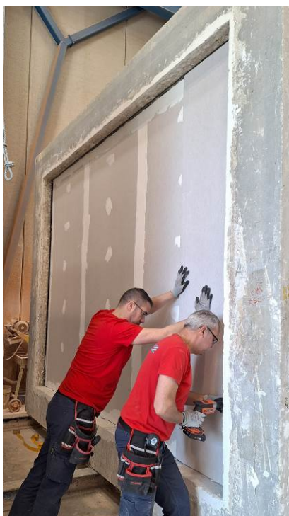
Photos of assembly of the test specimen
