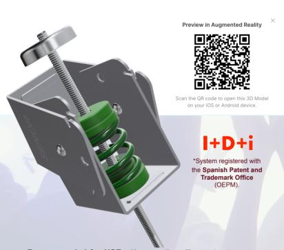
**Recommended for USE** with acoustic ceilings, structure suspensions, and machinery with an operational frequency above 350 RPM and a load ranging between 10 and 45 kg per support point.
