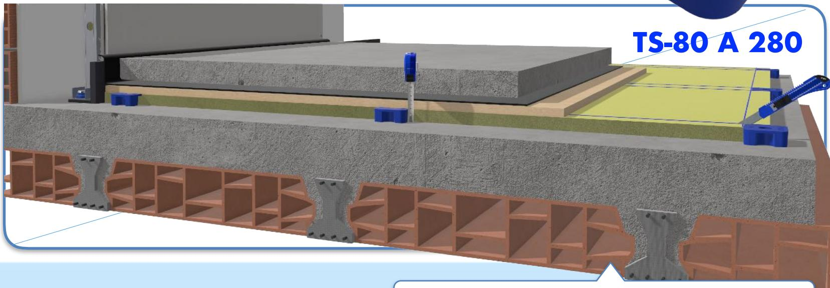
**Suggested use:** rubber mount for acoustic floors under **concrete slab**. This type of polymer has a better damping result than other rubbers such as polyurethane, polystyrene, EPDM, among others.
