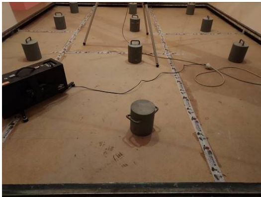
Photos of test specimen in the acoustic rooms Under load (left) and without loading (right)
