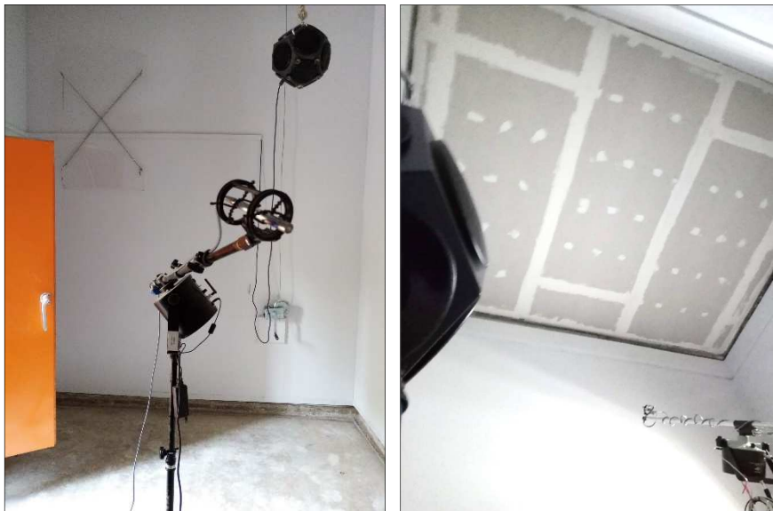
Images 28 and 29 Test specimen installed and ready for the test, view from source and receiving room
