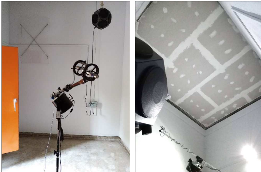
Images 22 and 23 Test specimen installed and ready for the test, view from source and receiving room
